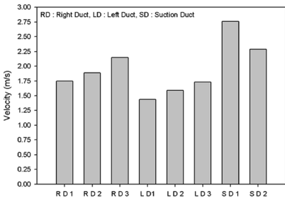
Fig. 10 Average velocity in inlet and outlet ducts
