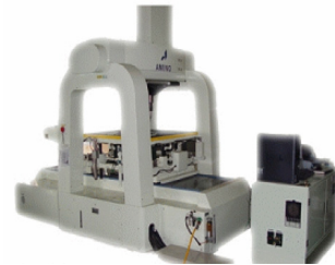
Fig. 4 Incremental forming machine(DLNC-PA)
