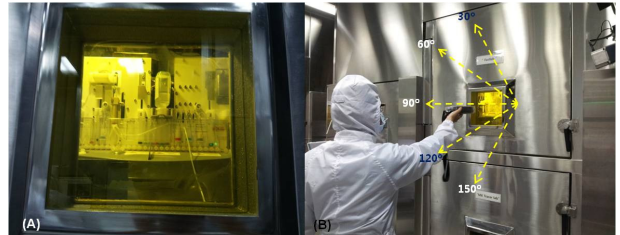
Fig.3 Measuring outside scatter ray of 18 F-FDG synthesis equipment in hot cell
