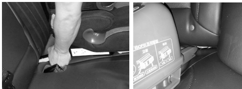
Fig. 5 Difficult low anchor access
