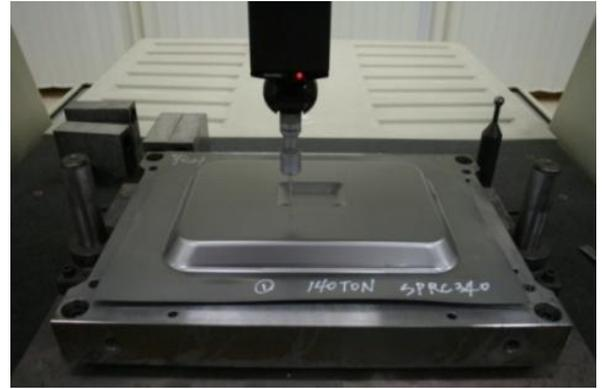
Fig. 11 Measurement of blank shape by CMM
