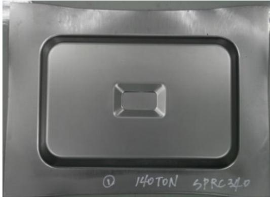
Fig. 9 Blank after forming
