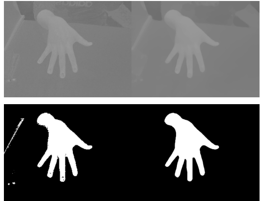
[Fig. 4] Result of the noise removal process using median filter
