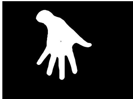
[Fig. 6] Result of a center point detection of hand using the distance transform matrix
