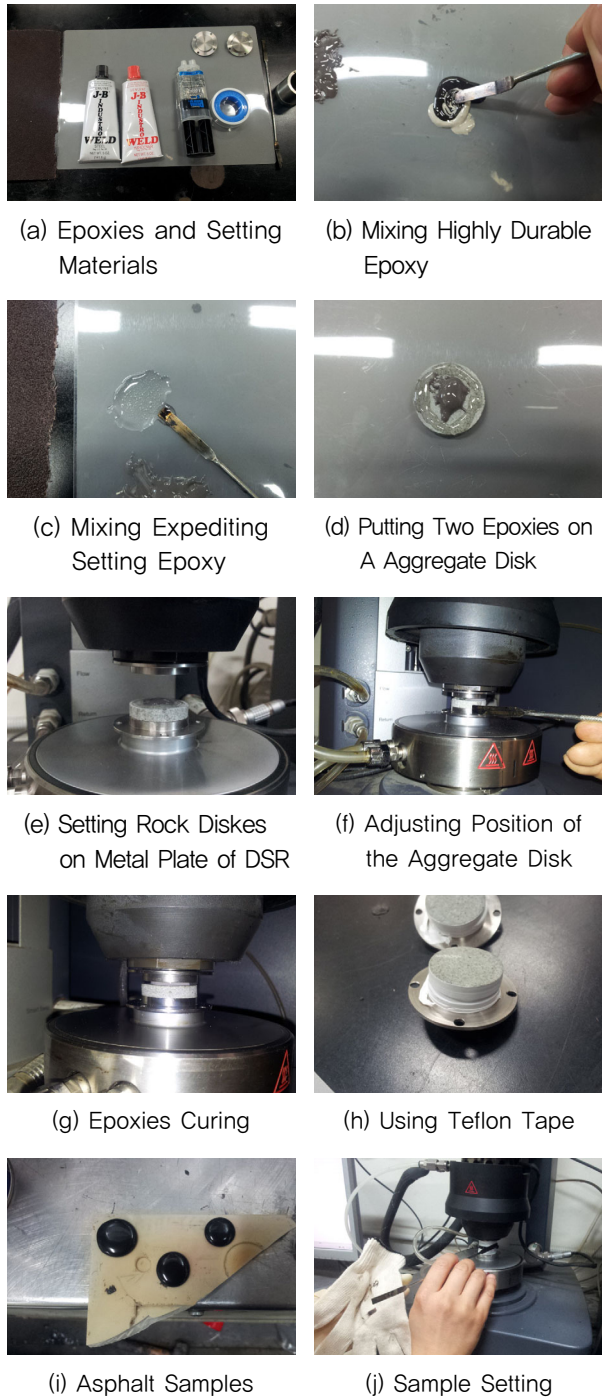
Fig. 5 Preparation of Stress Sweep using Rock Disks
