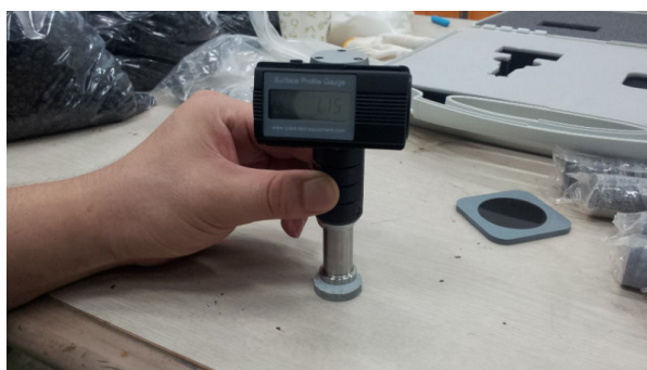
Fig. 3 Surface Profile Gauge to Measure Roughness
