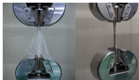
<Fig. 3> Reinforced component materials test (Left-Glass, Right-AL 6063 T6)
