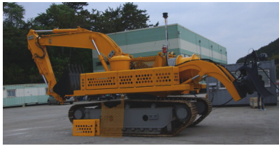
[Fig. 1] Underwater equipment for rubble mound leveling
