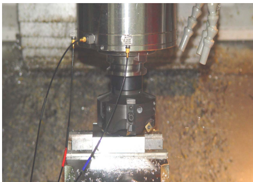
[Fig. 3] Photograph for vibration test of milling cutter
