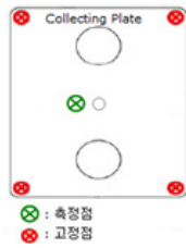
[Fig. 6] Measuring points on the collecting plate
