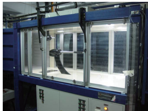
Fig. 3. Closed-circuit wind-tunnel test section with sting balance
