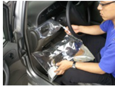
Fig. 3 Photo of VOCs collection by using GSB
