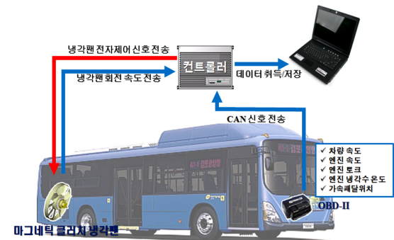
Fig. 6 Schematic of real road vehicle test
