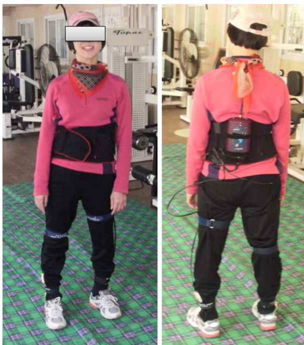
Figure 1. The front and rear view of the participant wearing the Pedar-X
