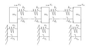
FIGURE 1. An n degree of freedom damped mass-spring system. [9]
