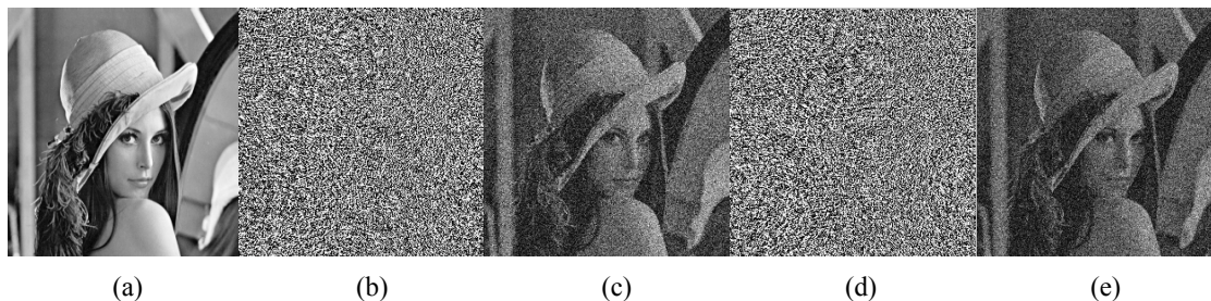
FIG. 8. (a) Original Lena image ( 256 \times 256 ), (b) Product of POF1 and POF3, (c) Reconstructed image from the product of POF1 and POF3, (d) Product of POF2 and POF3, (e) Reconstructed image from the product of POF2 and POF3.
