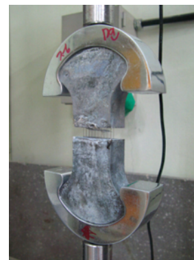
Fig. 3 Manufacturing of specimens for pullout test
