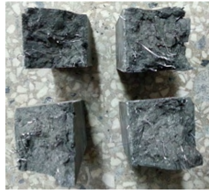
Fig. 3 Fiber ball in RPC specimens (B40 type)
