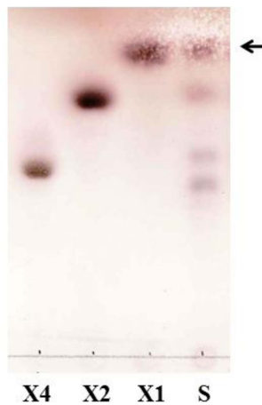
Fig. 4. Thin layer chromatogram of the hydrolyzed product of beechwood xylan by HX-1 xylanase.
