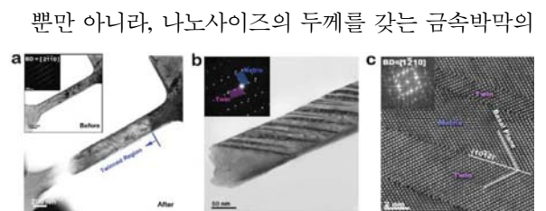
Fig. 8. TEM images from in situ tensile tests of [0001] oriented Mg. 17)
