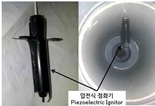
Fig. 3. Installation of piezoelectric ignitor in the combustion chamber
