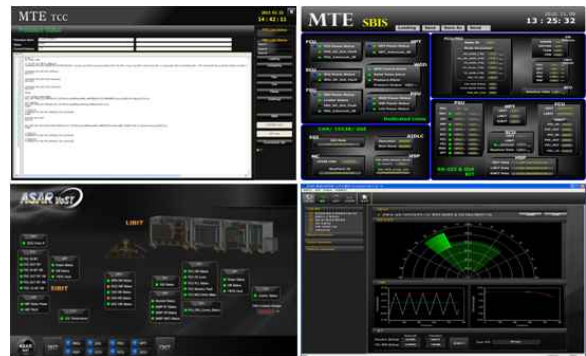
Fig. 4. SCCTE GUI: Script Execution(Left Top), SAR Unit Simulator(Right Top), SAR Telemetry(Left Bottom), GMTI Data Analysis(Right Bottom)
