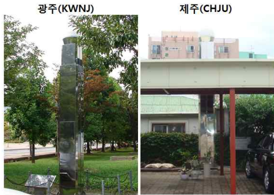
Fig. 1. Examples of Poorly Sited GNSS Stations in Gwangju and Jeju
