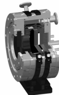
Fig. 2 Cross-sectional structure of the low-temperature vacuum blackbody
