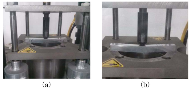
Fig. 9. Process of impact test for specimen: (a) Specimen underwent bending deformation, (b) Damage initiation and evolution in specimen.
