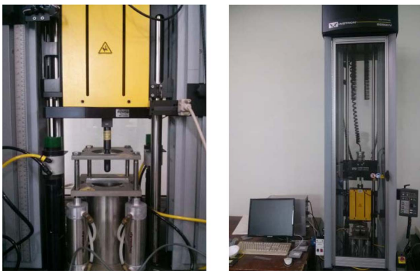
Fig. 3. Instron Dynatup® Impact Test Machine used in experiment.
