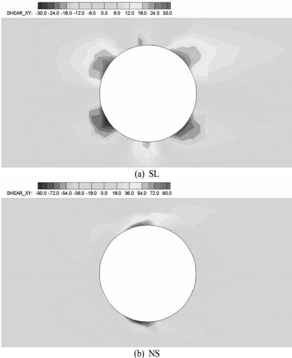
Fig. 11. Shear stress in xy-direction(Unit: N/m 2 ).
