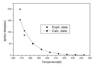
Fig. 2. A comparison between the experimental and calculated delay times for n-pentadecane.
