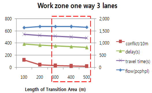
Figure 6. The conflict/10m, delay, travel time, and flow according to the length of transition area
