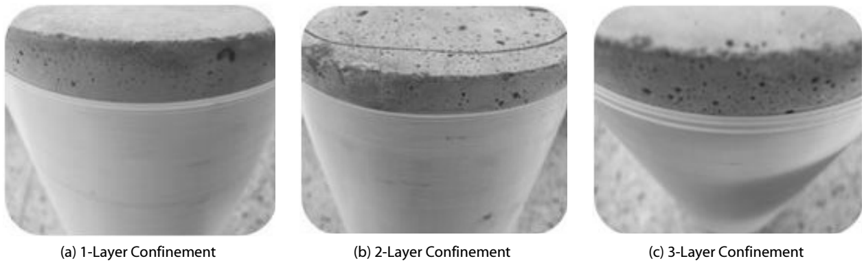
Fig. 3. Concrete Cylinders Confined with FRP Wire
