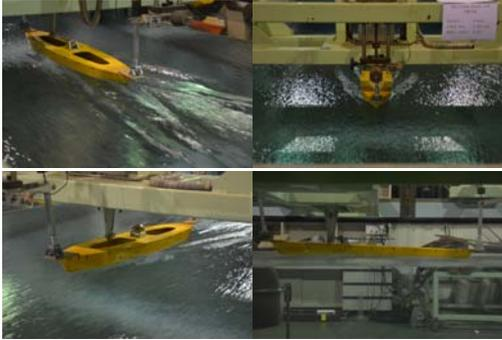
Figure 6: Photographs of Resistance Test (RD-FK-11) : 6.0 knots
