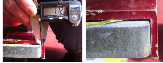
Figure 1: Plasma cutting plane phenomenon
