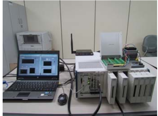
Figure 3: Hardware components of HIL Simulator
