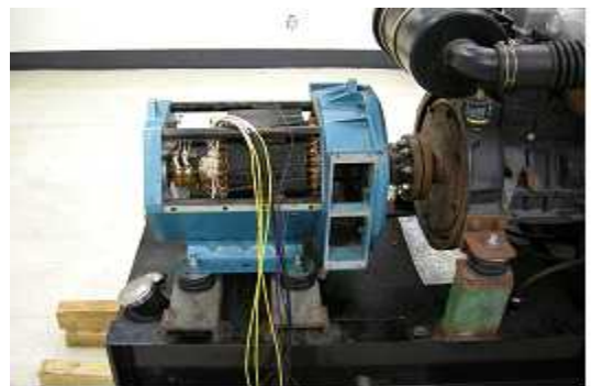
Figure 6: 2 pole synchronous generator for fault test
