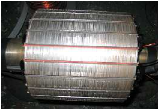
Figure 4: Rotor for synchronous generator
