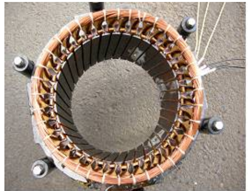
Figure 2: Stator for synchronous generator
