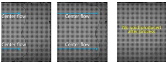
Figure 10: Movement of meniscus at the bump pitch 80 \mu\text{m} in the rectangular array; (a) the early flow fronts, (b) the final flow fronts, (c) no void produced after the filling process
