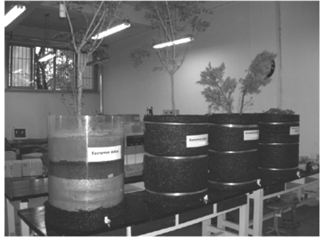
Figure 2. Pilot-scaled bio-retention experimental reactor.
