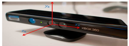
Fig. 14 Kinect coordinate system
