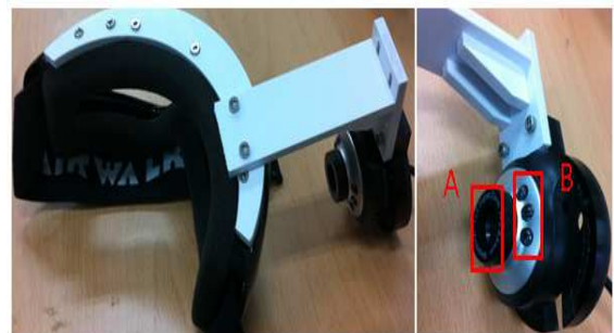
Fig. 5 Camera and infrared light for Gaze tracking
