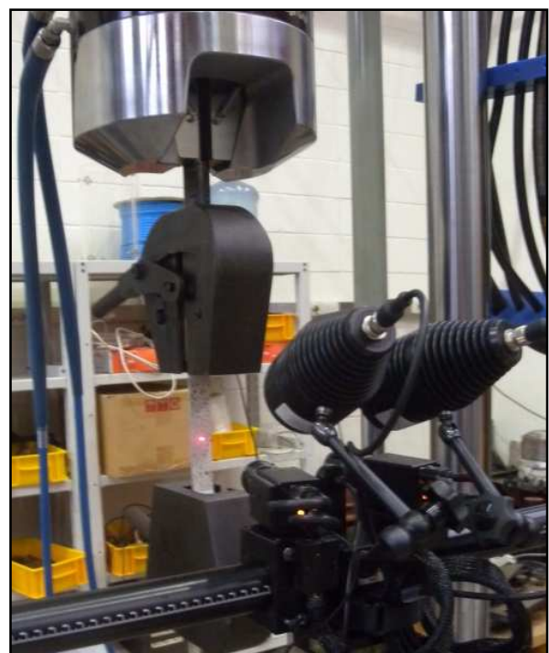
Fig. 4 Photograph for tensile testing system and strain measurement system
