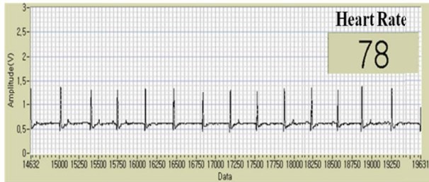
Fig. 2. Electrocardiogram data sent from the sensor node and heart rate calculated with LabVIEW.
