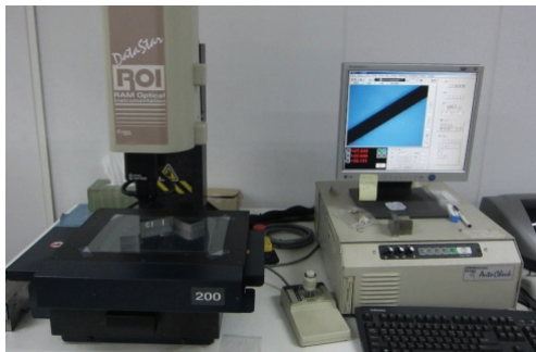
Fig. 8 Measurement of three-dimensional shape of the fabricated prototypes
