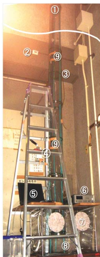
Fig. 1. Experimental set up to study the scavenging of dust particles by rainfall.
