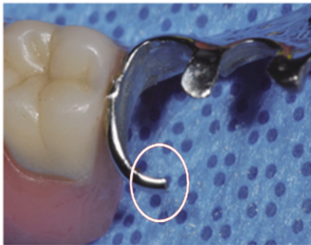
Fig. 4. Fracture of Aker's clasp by fatigue failure.
