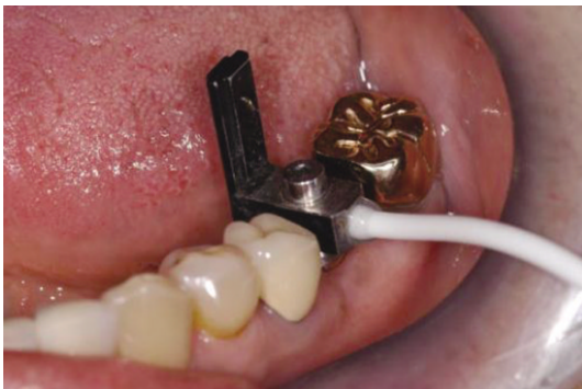
Fig. 1. A transducer (Type A1) connection onto implant fixture.
