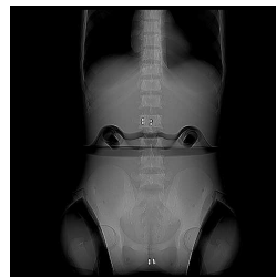
[Fig. 3] CT image of Humanoid phantom showing the location of the Glass Rod Detector at the level of the pelvis.
