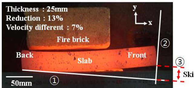
Fig. 3 Side view of material in which the ski is formed after the rolling test
