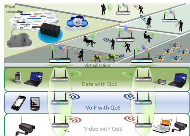
Fig. 3. Virtual network environment. QoS: quality of service, VoIP: voice over Internet protocol.
