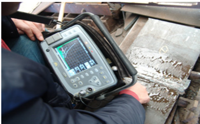
Fig. 8 Nondestructive weld examination
