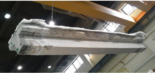
Fig. 8 Test result of spray-on fire protection
