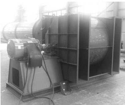
Fig. 1 Double-inlet centrifugal blower
