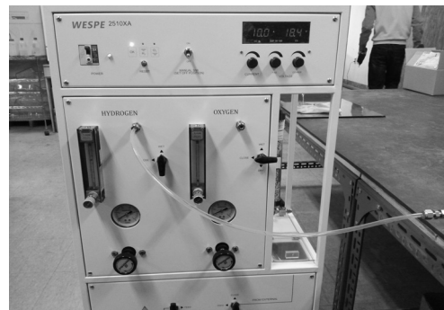
Fig. 5 P.E.M Type electrolyser made by WESPE 8)
